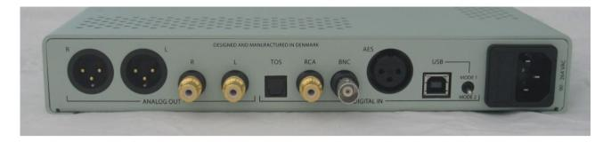
**Analog Out:** The dac1541 have balanced line out using 3 pins XLR sockets, marked "R" for the right channel and "L" for the left channel. It also have single ended line out using RCA sockets, the red one marked "R" is for the right channel, the white one marked "L" is for the left channel.
