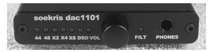
The LED's indicates input sample rate, volume level and anti-aliasing filters selected.
