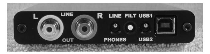
The two RCA Phone sockets are for line out signal, the white one marked "L" is for the left channel, the red one marked "R" is for the right channel.
